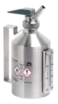
Stainless steel 1.4571 (AISI 316Ti) polished Dimensions: approx. 100 x 210 mm (dia x H) without srew cap. Flame arrester in container neck, Level control via integrated sight glass with measuring scale. Markin prepared according to GefStoffV including self-closing metering tap with seal of PTFE. Open by pushing or pulling. Self-closing prevents uncontrolled leakage of liquids. Setting ring for adjustment, afeter installation vertically adjustable.
