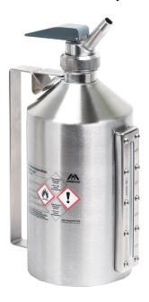
Stainless steel 1.4571 (AISI 316Ti) polished Dimensions: approx. 115 x 305 mm (dia x H) without srew cap. Flame arrester in container neck, Level control via integrated sight glass with measuring scale. Markin prepared according to GefStoffV including self-closing metering tap with seal of PTFE. Open by pushing or pulling. Self-closing prevents uncontrolled leakage of liquids. Setting ring for adjustment, afeter installation vertically adjustable.
