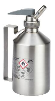
Stainless steel 1.4571 (AISI 316Ti) polished Dimensions: approx. 100 x 210 mm (dia x H) without srew cap. Flame arrester in container neck, Markings prepared according to GefStoffV and Workplace Directive A1.3 (ASR). Including self-closing, with seal of PTFE. Opens by pushing or pulling. Self-closing prevents uncontrolled leakage of liquids. Setting ring for adjustment, after installation vertically adjustable.
