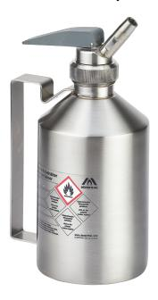
Stainless steel 1.4571 (AISI 316Ti) polished Dimensions: approx. 100 x 210 mm (dia x H) without srew cap. Flame arrester in container neck, Markings prepared according to GefStoffV and Workplace Directive A1.3 (ASR). Including self-closing, with seal of PTFE. Opens by pushing or pulling. Self-closing prevents uncontrolled leakage of liquids. Setting ring for adjustment, after installation vertically adjustable.
