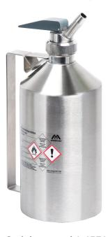
Stainless steel 1.4571 (AISI 316Ti) polished Dimensions: approx. 115  $\times$  305 mm (dia  $\times$  H) without srew cap. Flame arrester in container neck, Markin prepared according to GefStoffV including self-closing metering tap with seal of PTFE. Open by pushing or pulling. Self-closing prevents uncontrolled leakage of liquids. Setting ring for adjustment, afeter installation vertically adjustable.
