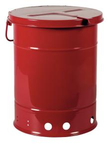
Capacity 20 I, Dim: 290 x 397 (dia x H mm), sheet steel, exterior red powder coated, interior tinplated, self-closing lid, opening by hand, Markings prepared according to GefStoffV and BGV A8 testing: GS-sign and FM/UL-tested
