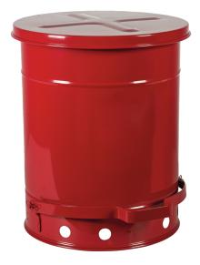
Dim:approx.  $348 \times 458$  (dia x H mm), sheet steel, exterior red powder coated, interior tin-plated, self-closing lid, using foot pedal for opening, Markings prepared according to GefStoffV and BGV A8 testing: FM/UL-tested
