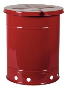
Capacity 40 I, Dim:  $348 \times 458$  (dia x H mm), sheet steel, exterior red powder coated, interior tinplated, self-closing lid, opening by hand, Markings prepared according to GefStoffV and BGV A8 testing: FM/UL-tested
