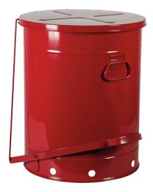
Dim:approx. 458 x 597 (dia x H mm), sheet steel, exterior red powder coated, interior tin-plated, self-closing lid, using foot pedal for opening, Markings prepared according to GefStoffV and BGV A8 testing: FM/UL-tested
