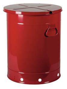
Capacity 80 I, Dim: 458 x 597 (dia x H mm), sheet steel, exterior red powder coated, interior tinplated, self-closing lid, opening by hand, Markings prepared according to GefStoffV and BGV A8 testing: FM/UL-tested
