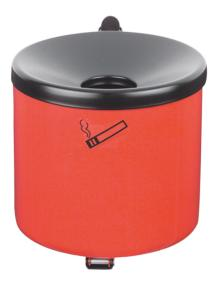
Safety wall ashtray made from sheet steel Container powder-coated, red Chute painted, black Dim. ( $\emptyset \times H$ ) approx. 150 x 145 mm Capacity: 2,4 I Funnel-formed lid opening prevents supply of oxgen in case of fire. Due to the construction of the extinguishing head smouldering cigarette butts are automatically extinguished, easy disposal, with wall bracket.
