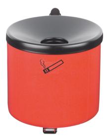
Safety wall ashtray made from sheet steel Container powder-coated, red Chute painted, black Dim. ( $\emptyset$  x H) approx. 150 x 145 mm Capacity: 2,4 I Funnel-formed lid opening prevents supply of oxgen in case of fire. Due to the construction of the extinguishing head smouldering cigarette butts are automatically extinguished, easy disposal, with wall bracket.
