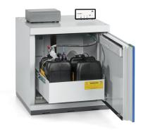
Classical door technology (push-to-open), door hinge right. For the active storage of flammable liquids. type testing by MPA/TÜV SÜD according to DIN EN 14470-1, DIN EN 14727, EK5/AK4 21-01:2021 and AfPS GS 2019: 01 PAK. Classification of ex-zones according to DIN EN 60079-10. Mark of approval: GS/CE mark, high quality mark of approval by TÜV SÜD. Construction and colour:
