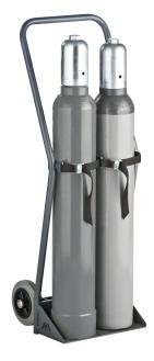
Suitable for the transport of 2 x 10 litre gas cylinders. With solid rubber tyres. Load bearing capacity: 100 kg. Colour: RAL 7015, coarse structure. Size appropriate for the storage in safety cabinets for gas cylinders: models SUPREME plus M,L,XL,XXL as well as models ECO plus M,L,XL,XXL and gas cylinder depots M,L,XL, Dimensions (W x D x H) approx.: 356 x 317 x 1000 mm
