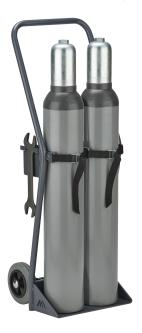
Suitable for the transport of 2 x 10 litre gas cylinders. With solid rubber tyres. Load bearing capacity: 100 kg. Including toolbox and wrench SW 30/32. Colour: RAL 7015, coarse structure. Size appropriate for the storage in safety cabinets for gas cylinders: models SUPREME plus M,L,XL,XXL as well as models ECO plus M,L,XL,XXL and gas cylinder depots M,L,XL, Dimensions (W x D x H) approx.: 356 x 317 x 1000 mm
