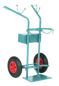
With solid rubber tyres. Suitable for the transport of 2 x 50 litre gas cylinders. Blue painted steel tube construction. Including securing chain. With lockable toolbox. Dimensions (W x D x H) approx.: 770 x 780 x 1350 mm
