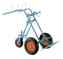
With solid rubber tyres and fold-out tail wheel. Suitable for the transport of 2 x 50 litre gas cylinders. Blue painted steel tube construction. Including securing chain. Finger guards for safe grip. Dimensions (W x D x H) approx.:  $770 \times 800 \times 1350$  mm
