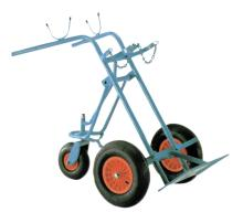
With solid rubber tyres and fold-out tail wheel. Suitable for the transport of 2 x 50 litre gas cylinders. Blue painted steel tube construction. Including securing chain. Finger guards for safe grip. With lockable toolbox, large hose and torch holder and two welding rod holders. Dimensions (W x D x H) approx.:  $770 \times 800 \times 1600 \text{ mm}$
