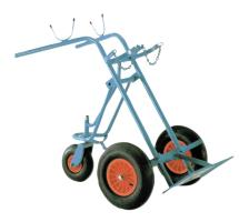
With solid rubber tyres and fold-out tail wheel. Suitable for the transport of 2 x 50 litre gas cylinders. Blue painted steel tube construction. Including securing chain. Finger guards for safe grip. With lockable toolbox, large hose and torch holder and two welding rod holders. Dimensions (W x D x H) approx.: 770 x 800 x 1600 mm
