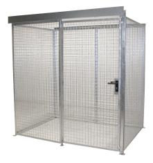
for 48 gas cylinders dia = 220 mm For outdoor storage of gas cylinders in accordance with the regulations. surface hot-dip galvanised according to EN ISO1461 delivery in modular system with assembly instructions for self-assembly dimensions (outside) in mm:  $2100 \times 1500 \times 2180$  (WxDxH) Design according to TRGS 510.
