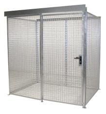
for 48 gas cylinders dia = 220 mm For outdoor storage of gas cylinders in accordance with the regulations. surface hot-dip galvanised according to EN ISO1461 delivery in modular system with assembly instructions for self-assembly dimensions (outside) in mm:  $2100 \times 1500 \times 2180$  (WxDxH) Design according to TRGS 510.
