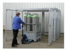
for 78 gas cylinders dia = 220 mm for outdoor storage of gas cylinders in accordance with the regulations. surface hot-dip galvanised according to EN ISO1461 delivery in modular system with assembly instructions for self-assembly incl. double wing door W x H 2160 x 1985 mm with profile cylinder dimensions (outside) in mm: 3100 x 1500 x 2160 (WxDxH) Design according to TRGS 510.
