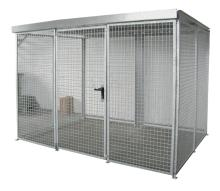
for 104 gas cylinders dia = 220 mm for outdoor storage of gas cylinders in accordance with the regulations. surface hot-dip galvanised according to EN ISO1461 delivery in modular system with assembly instructions for self-assembly dimensions (outside) in mm:  $3100 \times 2100 \times 2180$  (WxDxH) Design according to TRGS 510.
