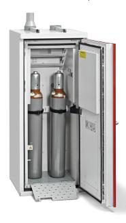
Classical door technology (door handle), door hung right. For the storage of pressurised gas cylinders. Type testing by MPA/TÜV SÜD according to DIN EN 14470-2, DIN EN 16121 and DIN EN 16122, EK5/AK4 09-10:2009 and AfPS GS 2014:01 PAK Mark of approval: GS/CE mark, high quality mark of approval by TÜV SÜD Construction and colour:
