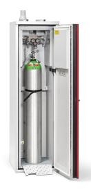
Classical door technology (door handle), door hung right. For the storage of pressurised gas cylinders. Type testing by MPA/TÜV SÜD according to DIN EN 14470-2, DIN EN 16121 and DIN EN 16122, EK5/AK4 09-10:2009 and AfPS GS 2014:01 PAK Mark of approval: GS/CE mark, high quality mark of approval by TÜV SÜD Construction and colour:
