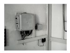
with hand-held terminal approved for zone 1 potentially explosive atmospheres Housing made from highly-resistant, impact-resistand polycarbon with 12 m cable. Dim. (WxDxH): approx. 280 x  $280 \times 160 \text{ mm}$  TÜV-proofed
