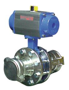
Material stainless steel, PTFE coating Cut-off flaps set consisting of: Flaps are supplied complete with pneumatic part-turn actuator Tanker couplings with dummy caps for threaded tapered union and connecting mother part and flanged threaded nipples, completely mounted.
