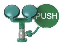
Stainless steel ball valve, not self-closing. Push plate made of steel, powder-coated in green. Water-bearing parts made of brass. Including emergency sign (pictogram). Water flow rate: 14 l/min. at 1.5 - 5 bar flow pressure, incl. automatic flow regulation. Required water connection: ½" internal thread. Tested acc. to: BGI/GUV-I 850-0, DIN 1988, DIN EN 1717, ANSI Z358.1-2004, DIN EN 15154-2. Tested and certified acc. to DIN-DVGW.
