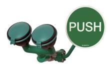
Stainless steel ball valve, not self-closing. Push plate made of steel, powder-coated in green. Water-bearing parts made of brass. Including emergency sign (pictogram). Shower heads 45° angled. Water flow rate: 14 l/min. at 1.5 - 5 bar flow pressure, incl. automatic flow regulation. Required water connection: ½" internal thread. Tested acc. to: BGI/GUV-I 850-0, DIN 1988, DIN EN 1717, ANSI Z358.1-2004, DIN EN 15154-2. Tested and certified acc. to DIN-DVGW.
