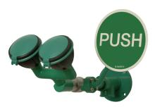
Stainless steel ball valve, not self-closing. Push plate made of steel, powder-coated in green. Water-bearing parts made of brass. Including emergency sign (pictogram). Shower heads 45° angled. Water flow rate: 14 l/min. at 1.5 - 5 bar flow pressure, incl. automatic flow regulation. "Required water connection: 3/4"" external thread." Tested acc. to: BGI/GUV-I 850-0, DIN 1988, DIN EN 1717, ANSI Z358.1-2004, DIN EN 15154-2. Tested and certified acc. to DIN-DVGW.
