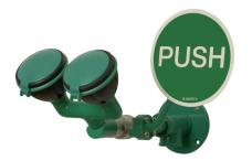
Stainless steel ball valve, not self-closing. Push plate made of steel, powder-coated in green. Water-bearing parts made of brass. Including emergency sign (pictogram). Shower heads 45° angled. Water flow rate: 14 I/min. at 1.5 - 5 bar flow pressure, incl. automatic flow regulation. "Required water connection: 3/4"" external thread." Tested acc. to: BGI/GUV-I 850-0, DIN 1988, DIN EN 1717, ANSI Z358.1-2004, DIN EN 15154-2. Tested and certified acc. to DIN-DVGW.
