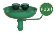
Stainless steel ball valve, not self-closing. Collecting basin made of stainless steel, powder-coated in green. Push plate made of steel, powder-coated in green. Water-bearing parts made of brass. Including emergency sign (pictogram). Water flow rate: 16 l/min. at 1.5 - 5 bar pressure, incl. automatic flow regulation. Required water connection: 3/4" external thread. Tested acc. to: BGI/GUV-I 850-0, DIN 1988, DIN EN 1717, ANSI Z358.1-2004, DIN EN 15154-2. Tested and certified acc. to DIN-DVGW.
