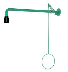
Shower arm made of brass, powder-coated in green. Stainless steel ball valve. High-performance shower head made of chemical-resistant plastic, self-draining. Including emergency sign (pictogram). Water flow rate: 50 l/min. at 1.5 - 3 bar flow pressure, incl. automatic flow regulation. Required water connection: <sup>3</sup>/<sub>4</sub>" external thread. Tested acc. to: BGI/GUV-I 850-0, DIN 1988, DIN EN 1717, ANSI Z358.1-2004, DIN EN 15154-1. Tested and certified acc. to DIN-DVGW.
