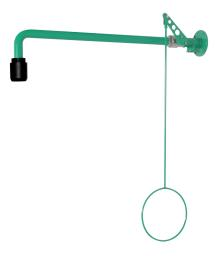
Shower arm made of brass, powder-coated in green. Stainless steel ball valve. High-performance shower head made of chemical-resistant plastic, self-draining. Including emergency sign (pictogram). Water flow rate: 50 l/min. at 1.5 - 3 bar flow pressure, incl. automatic flow regulation. Required water connection: <sup>3</sup>/<sub>4</sub>" external thread. Tested acc. to: BGl/GUV-I 850-0, DIN 1988, DIN EN 1717, ANSI Z358.1-2004, DIN EN 15154-1. Tested and certified acc. to DIN-DVGW.
