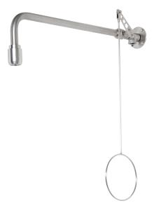
Shower arm, ball valve and pull rod made of stainless steel. High-performance shower head made of stainless steel, self-draining. Including emergency sign (pictogram). Water flow rate: 50 l/min. at 1.5 - 3 bar flow pressure, incl. automatic flow regulation. Required water connection: ¾" external thread. Tested acc. to BGI/GUV-I 850-0, DIN 1988, DIN EN 1717, ANSI Z358.1-2004, DIN EN 15154-1. Tested and certified acc. to DIN-DVGW.
