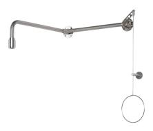
Piping, shower arm, ball valve and pull rod made of stainless steel. High-performance shower head made of stainless steel, self-draining. Including emergency sign (pictogram). Water flow rate: 50 l/min. at 1.5 - 3 bar flow pressure, incl. automatic flow regulation. Required water connection: <sup>3</sup>/<sub>4</sub>'' internal thread. Tested acc. to BGI/GUV-I 850-0, DIN 1988, DIN EN 1717, ANSI Z358.1-2004, DIN EN 15154-1. Tested and certified acc. to DIN-DVGW.
