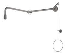
Piping, shower arm, ball valve and pull rod made of stainless steel. High-performance shower head made of stainless steel, self-draining. Including emergency sign (pictogram). Water flow rate: 50 l/min. at 1.5 - 3 bar flow pressure, incl. automatic flow regulation. Required water connection: <sup>3</sup>/<sub>4</sub>" internal thread. Tested acc. to BGI/GUV-I 850-0, DIN 1988, DIN EN 1717, ANSI Z358.1-2004, DIN EN 15154-1. Tested and certified acc. to DIN-DVGW.
